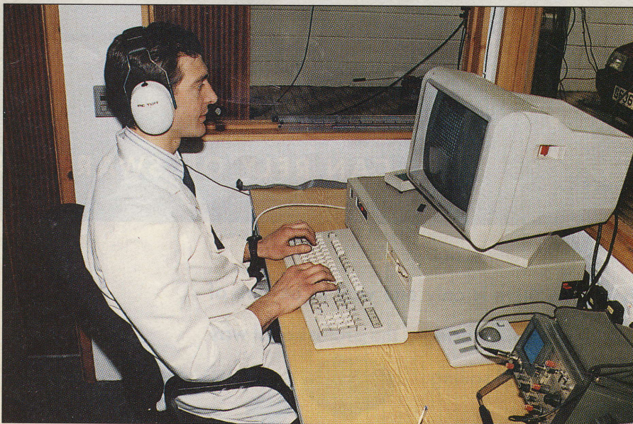
This computer is used to read chips and alter the programming they contain.
